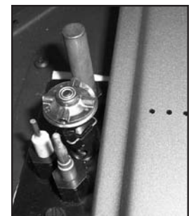
Figure 11. Ignitor assembly beside the burner.
